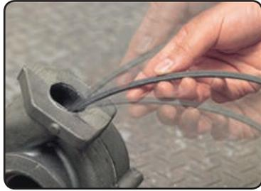
Our Video-probe is equipped with the latest technology in borescopes. A long fibre-optic cable illuminates the inspection area with light generated by a new state-of-the-art lamp in the Light Box. A miniature camera assembly in the viewing tip of the probe then converts the optical image into an electronic image. This image is carried back through the probe cable and displayed in the LCD color monitor. It allows the inspection of surfaces inside narrow tubes or difficult-to-reach chambers.
