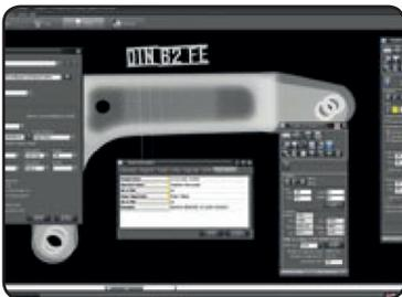
With film radiography the only variable is the film, with CR we have different IP's and the ability to adjust up to 4 parameters within the scanner to optimise the image quality to suit the required inspection task.
